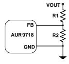
Figure 33. Setting the Output Voltage
