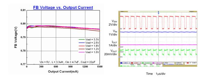
Figure 20. FB Voltage vs. Output Current
