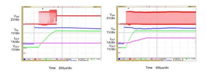
Figure 30. Soft Start Function (V<sub>IN</sub>=5V, V<sub>OUT</sub>=3.3V, I<sub>OUT</sub>=0A)
