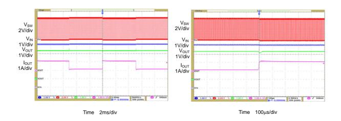
$\label{eq:figure 24. Dynamic Mode}$  (ILOAD=200mA to 1200mA, VIN=5V, VOUT=3.3V)
