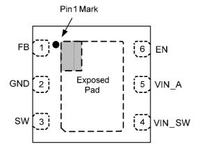
Figure 2. Pin Configuration of AUR9718 (Top View)
