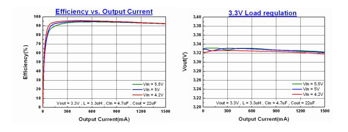
Figure 16. Efficiency vs. Output Current
