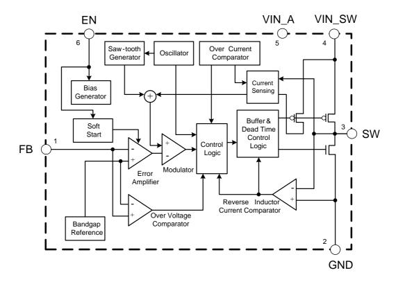
Figure 3. Functional Block Diagram of AUR9718
