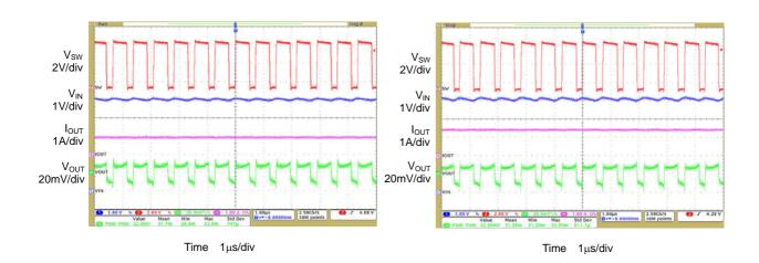
Figure 22.  $V_{OUT}$  Ripple ( $V_{IN}$ =5V,  $V_{OUT}$ =3.3V,  $I_{OUT}$ =1000mA)
