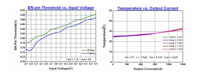
Figure 18. EN Pin Threshold vs. Input Voltage
