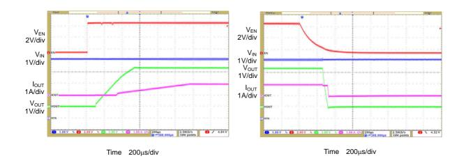
Figure 28. EN Pin L to H  $(V_{IN}=5V, V_{OUT}=3.3V, I_{OUT}=1A)$
