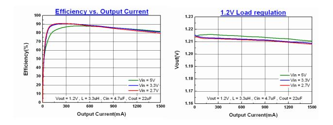
Figure 10. Efficiency vs. Output Current
