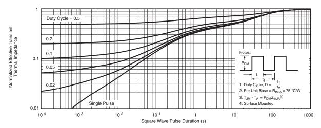
Normalized Thermal Transient Impedance, Junction-to-Ambient
