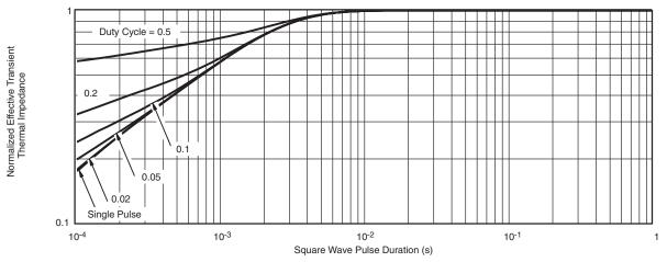
Normalized Thermal Transient Impedance, Junction-to-Case
