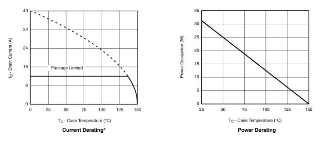
\* The power dissipation  $P_D$  is based on  $T_{J(max.)} = 150$  °C, using junction-to-case thermal resistance, and is more useful in settling the upper dissipation limit for cases where additional heatsinking is used. It is used to determine the current rating, when this rating falls below the package limit.
