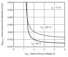
**On-Resistance vs. Gate-to-Source Voltage**
