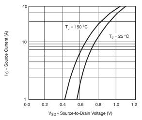
Source-Drain Diode Forward Voltage
