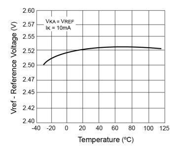
Figure 19: Reference Voltage vs. Temperature
