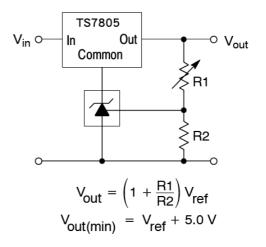
Figure 5: Output Control for Three Terminal Fixed Regulator
