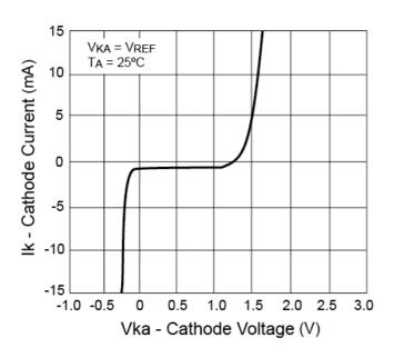
Figure 21: Cathode Current vs. Cathode Voltage
