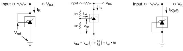
Figure 1:  $V_{KA} = V_{REF}$
