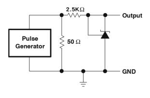
Test Circuit for Pulse Response, Ik=1mA
