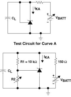
Test Circuit for Curve B, C and D
