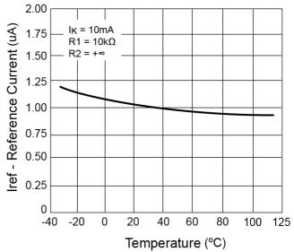
Figure 20: Reference Current vs. Temperature
