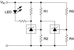
L.E.D. indicator is 'ON' when V<sub>in</sub> is between the upper and lower limits,
