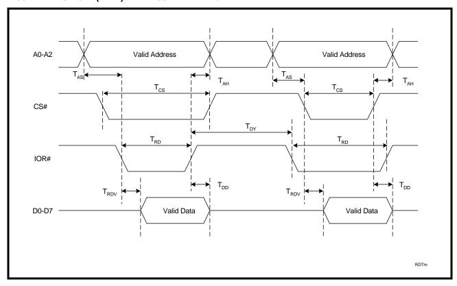
FIGURE 18. 16 MODE (INTEL) DATA BUS WRITE TIMING
