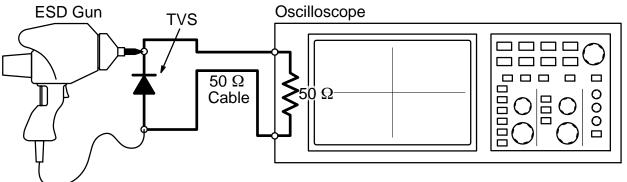
Figure 7. Diagram of ESD Test Setup
