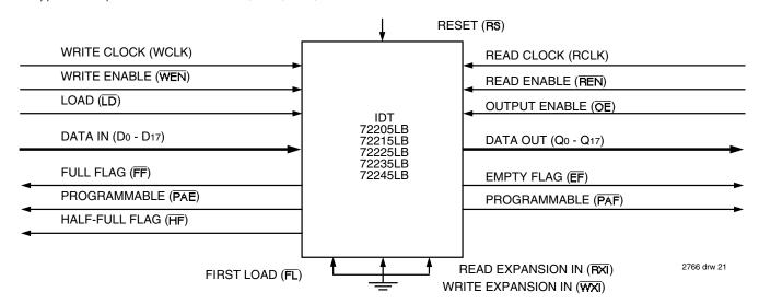
Figure 19. Block Diagram of Single 256 x 18, 512 x 18, 1,024 x 18, 2,048 x 18, 4,096 x 18 Synchronous FIFO
