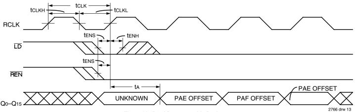
Figure 11. Read Programmable Registers
