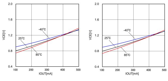
Figure 5 . Output Saturation Voltage2 vs Output Current
