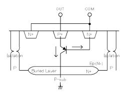
Figure 19. Construction of output clamp diode
