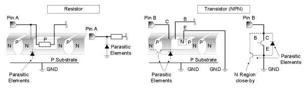
Figure 18. Example of monolithic IC structure
