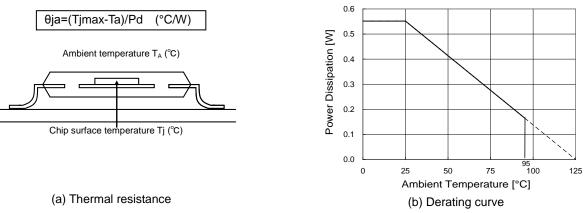
Figure 15. Thermal resistance and derating curve
