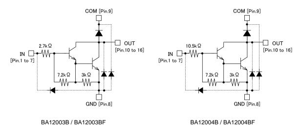
Note : The diode indicating the junction with a dotted line is a parasitic element. Note : The input and output parasitic diodes cannot be used as clamp diodes.
