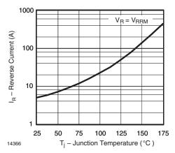
Fig. 2 - Max. Reverse Current vs. Junction Temperature
