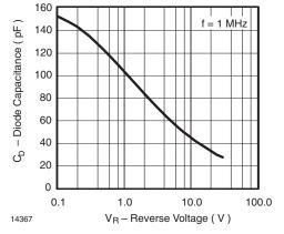
Fig. 5 - Typ. Diode Capacitance vs. Reverse Voltage
