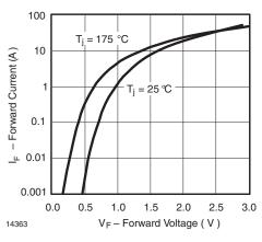
Fig. 4 - Max. Forward Current vs. Forward Voltage
