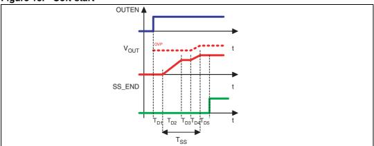
Once L6706 receives all the correct supplies and enables, it initiates the soft-start phase with a  $T_{D1}$  = 1.5 ms (typ) delay. After that, the reference ramps up to  $V_{BOOT}$  = 1.081 V (1.100 V - 19 mV) in  $T_{D2}$  according to the SSOSC settings and waits for  $T_{D3}$  = 200  $\mu$ sec (typ) during which the device reads the VID lines. Output voltage will then ramps up to the programmed value in  $T_{D4}$  with the same slope as before (*See Figure 13*).
