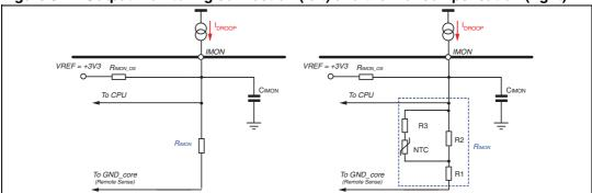
Current sense element (DCR inductor) has a non-negligible temperature variation. As a consequence, the sensed current is subjected to a measurement error that causes the monitoring voltage to vary accordingly.
