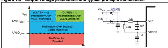
Figure 18. Output voltage protections and typical principle connections
