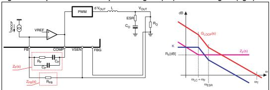
To obtain the desired shape an  $R_F$  -  $C_F$  series network is considered for the  $Z_F(s)$  implementation. A zero at  $\omega_F = 1/R_F C_F$  is then introduced together with an integrator. This integrator minimizes the static error while placing the zero  $\omega_F$  in correspondence with the L-C resonance assures a simple -20 dB/dec shape of the gain.
