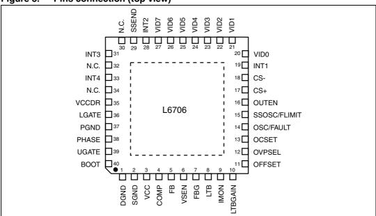
Figure 3. Pins connection (top view)
