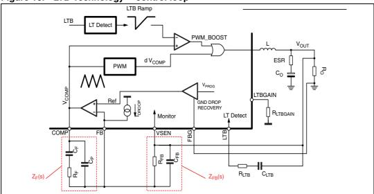
The LTB detector is able to detect output load transients by coupling the output voltage through an  $R_{LTB}$  -  $C_{LTB}$  network. After detecting a load transient, the LTB ramp is reset and then compared with the COMP pin level. The resulting duty-cycle programmed is then ORed with the PWM signal by-passing the main control loop. The phase will then be turned-on and the EA latencies results bypassed as well.
