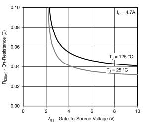
On-Resistance vs. Gate-to-Source Voltage
