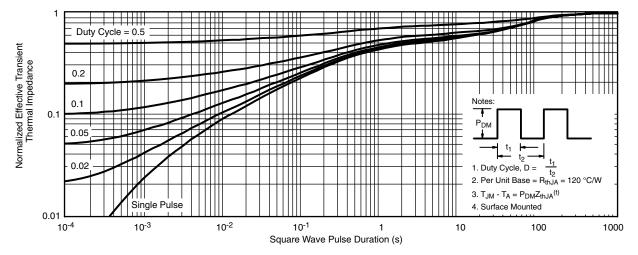
Normalized Thermal Transient Impedance, Junction-to-Ambient
