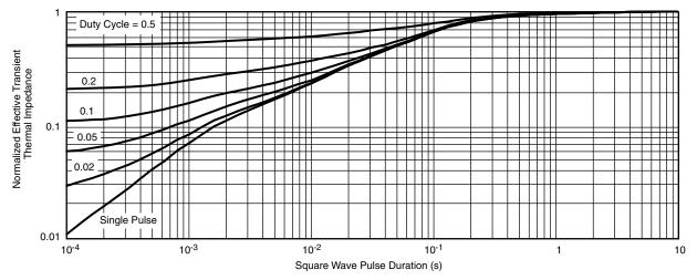
Normalized Thermal Transient Impedance, Junction-to-Foot
