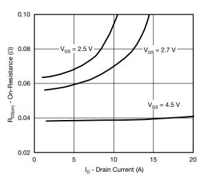
On-Resistance vs. Drain Current
