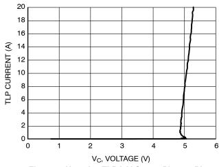
Figure 4. Negative TLP I-V Curve, Pin 1 to Pin 2
