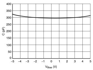
Figure 7. CV Characteristics
