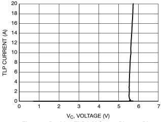
Figure 3. Positive TLP I-V Curve, Pin 2 to Pin 1
