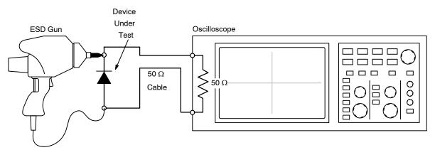
Figure 11. Diagram of ESD Test Setup
