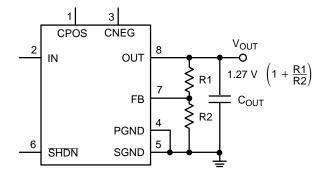
Figure 17. Programming the Adjustable CAT3200
