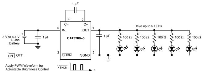
Figure 20. Lithium-Ion Battery to 5 V White or Blue LED Driver
