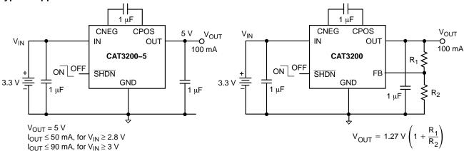
Figure 1. Typical Application - 5 V Output
