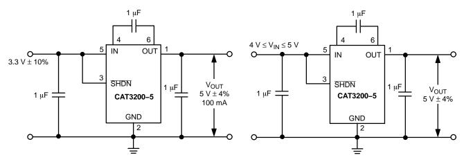
Figure 18. 3.3 V Supply to 5 V
