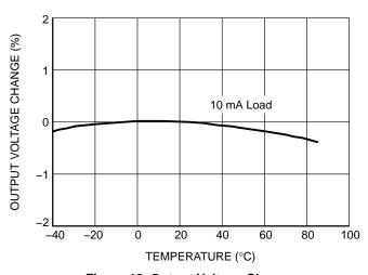
Figure 13. Output Voltage Change vs. Temperature
