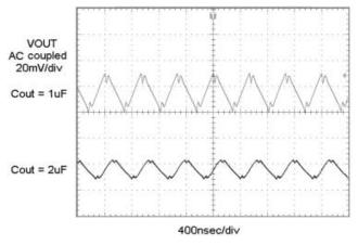
Figure 11. Output Ripple (100 mA Load, 3.3 V Input)
