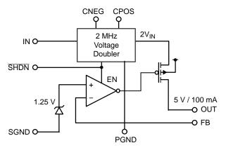
Figure 15. CAT3200 Adjustable Output
