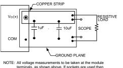
terminals, as shown above. If sockets are used then Kelvin connections are required at the module terminals to avoid measurement errors due to socket contact resistance
