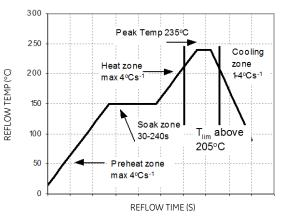
Figure 34. Reflow Profile for Tin/Lead (Sn/Pb) process.
