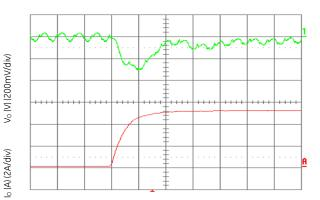
TIME, t (5  $\mu$ s/div) Figure 10. Transient Response to Dynamic Load Change from 50% to 100% of full load (Vo = 3.3Vdc).
