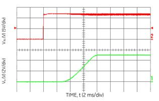
Figure 16. Typical Start-Up with application of Vin with low-ESR polymer capacitors at the output (7x150  $\mu$ F) (Vin = 12Vdc, Vo = 5.0Vdc, Io = 10A, Co = 1050  $\mu$ F)
