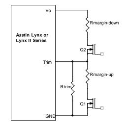
Figure 29. Circuit Configuration for margining Output voltage.
