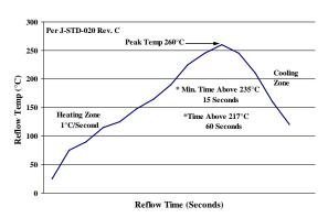
Figure 36. Recommended linear reflow profile using Sn/Ag/Cu solder.
