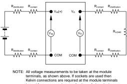
to avoid measurement errors due to socket contact resistance
