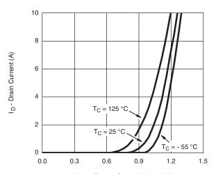
$V_{GS}$  - Gate-to-Source Voltage (V)
