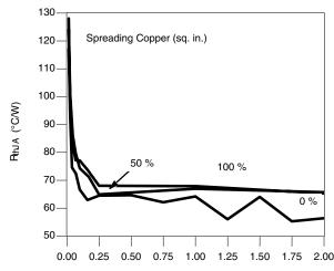
Figure 6. Spreading Copper - Junction-to-Ambient Performance
