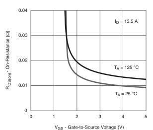
On-Resistance vs. Gate-to-Source Voltage
