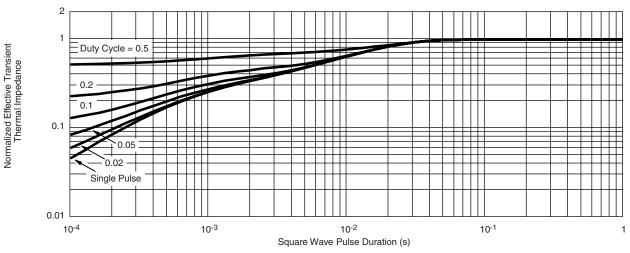
Normalized Thermal Transient Impedance, Junction-to-Case
