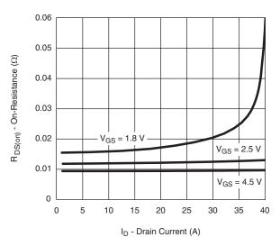
On-Resistance vs. Drain Current and Gate Voltage
